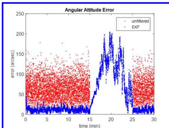
**Figure 5** – Attitude knowledge error as a function of time for the six-state MEKF, including a simulated star tracker anomaly.
