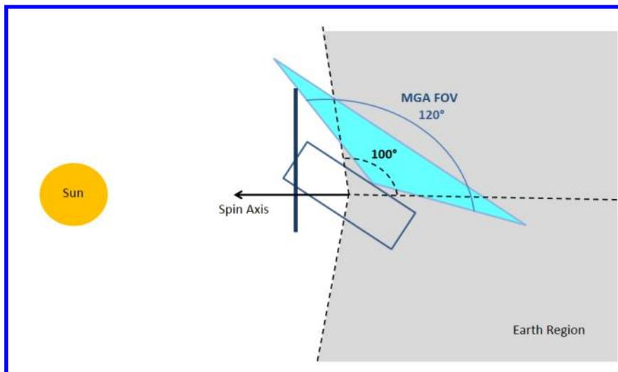
**Figure 13** – Geometry of the BioSentinel safe mode.
