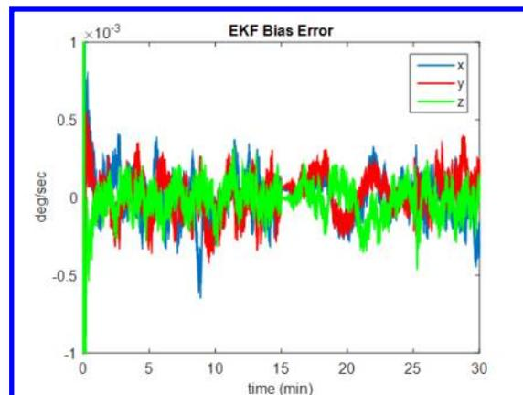
**Figure 6** – Gyro bias estimate as a function of time for the six-state MEKF used on BioSentinel.
