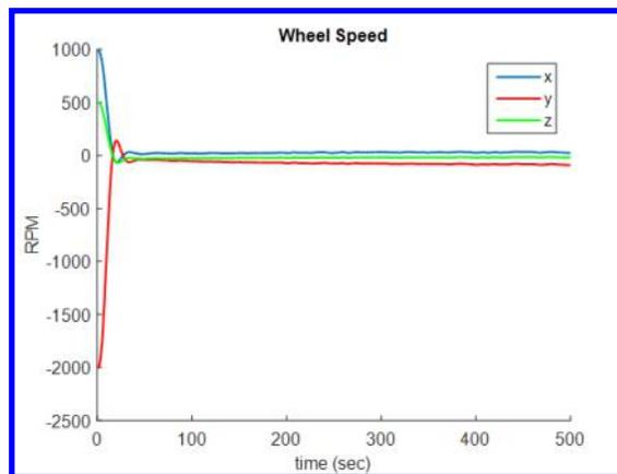
**Figure 10** – Wheel speed as a function of time during a momentum dump operation.
