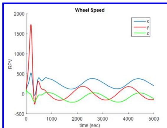
**Figure 15** – Wheel speed as a function of time using the safe mode controller.
