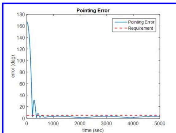
**Figure 14** – Pointing error as a function of time using the safe mode controller.
