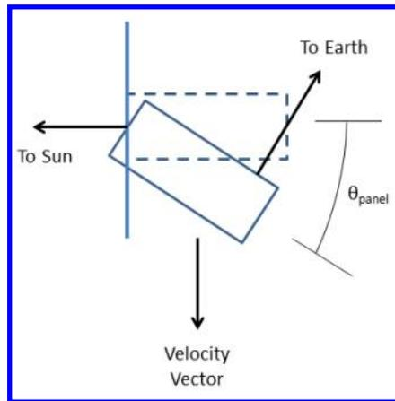
**Figure 7** – Geometry of the nominal operating mode used by the BioSentinel spacecraft.
