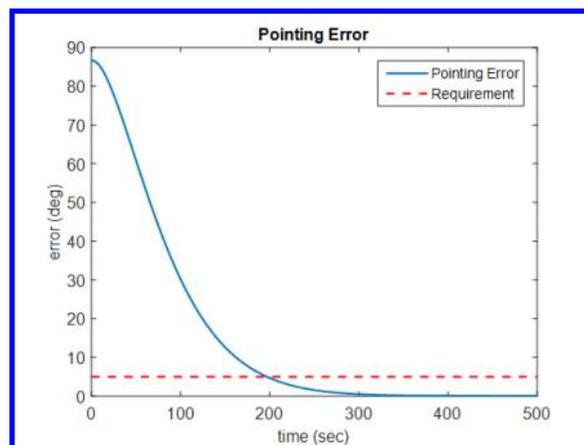
**Figure 8** – Pointing error as a function of time for a pointing maneuver undertaken during nominal spacecraft operations.
