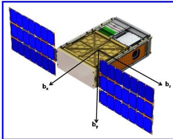
**Figure 2** – Artist’s depiction of the BioSentinel spacecraft, shown with solar panels deployed and one side panel removed.
