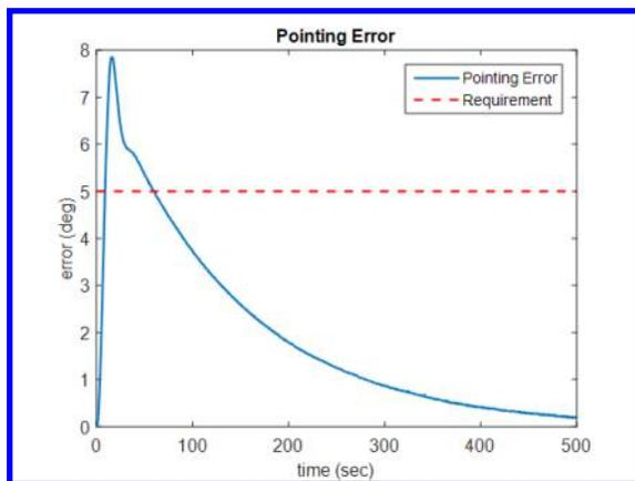
**Figure 9** – Pointing error resulting from a momentum dump operation during nominal mode.
