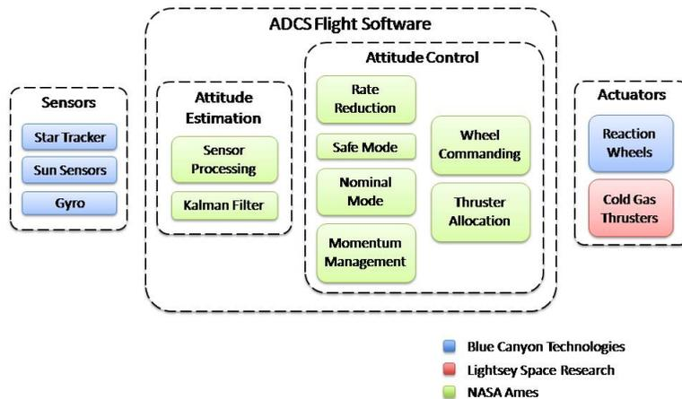
**Figure 3** – A block diagram representation of the attitude determination and control subsystem for the BioSentinel spacecraft.
