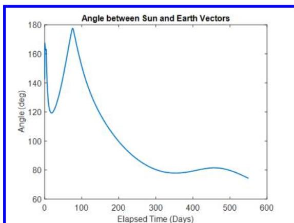
**Figure 11** – Angle between the Earth and the Sun relative to the BioSentinel spacecraft over the life of the mission.
