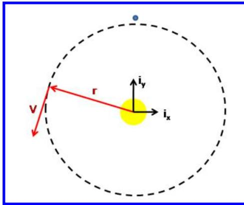
**Figure 4** – The Orbit frame is designed as a function of the position vector from BioSentinel to the sun  $\bar{r}$  and the spacecraft velocity vector  $\bar{V}$ .
