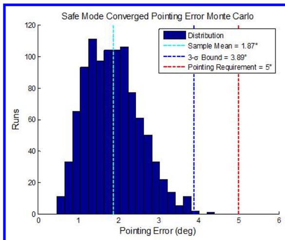
**Figure 16** – Results from the Monte Carlo analysis carried out to study the robustness of the safe mode controller used for the BioSentinel mission.
