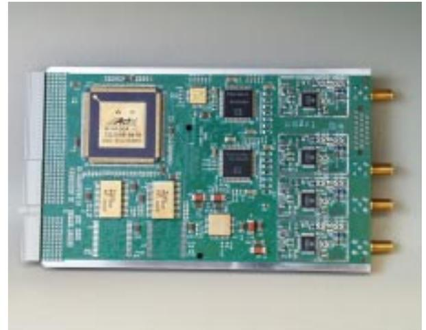
Fig. 3. PiVoT Receiver Engineering Model (courtesy of NASA Goddard Space Flight Center)
