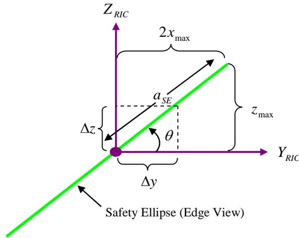
**Figure 8 – In-track-Cross-Track View of the Safety Ellipse, Edge-On**
