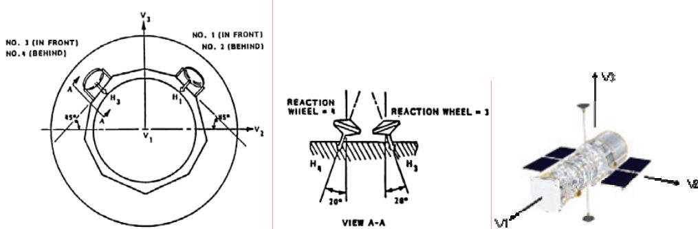
**Figure 1 Reaction wheel assembly configuration**
