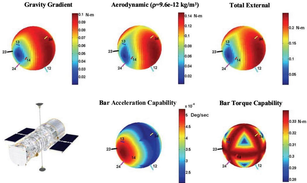
**Figure 2 External torque and MTB capability distribution**
