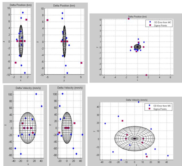
**Figure 7.** Different views of the position sigma points (top 3 plots) and the velocity sigma points (bottom 3 plots) relative to the formal OD covariance obtained from the OD process.
