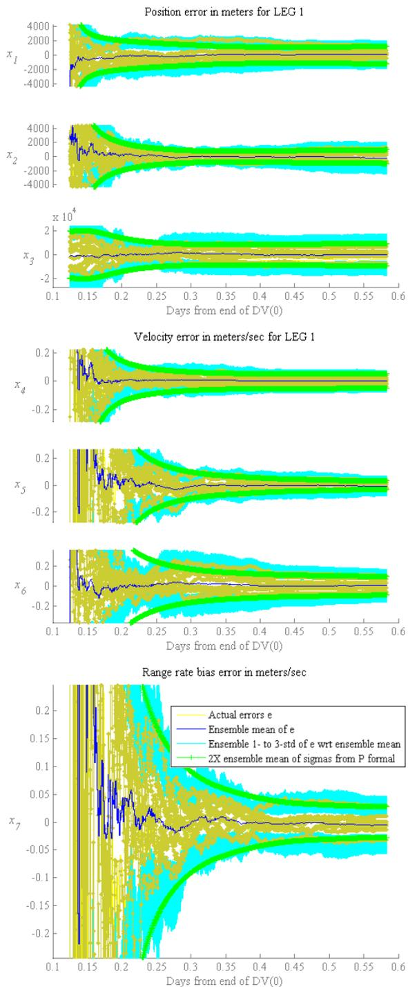
**Figure 6.** State estimation errors, their formal covariances, and the ensemble mean covariances from a 10-case Monte Carlo simulation of the Pre-Flyby OD. The dark solid line in each plot is the ensemble mean of all the estimate error.
