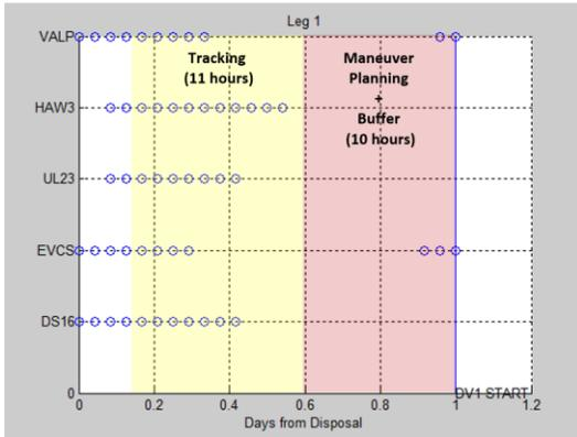
**Figure 5.** Station visibility at 1-hour increments
