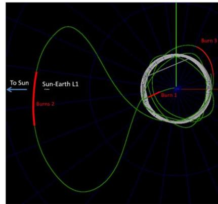
**Figure 1.** Nominal low-energy transfer trajectory
