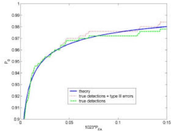
Figure 6: ROC for 10/10 integration, 25dB-Hz signal  $\omega = 0$  known,  $\tau$  unknown,  $P_{\text{FA}}$  divided down by 1023
