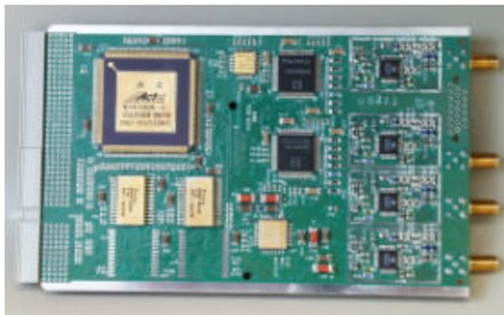
Figure 1: The PiVoT GPS Receiver
