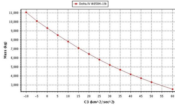
**Figure 4. Launch payload mass performance for the Boeing Delta-IV Heavy<sup>†</sup>.**
