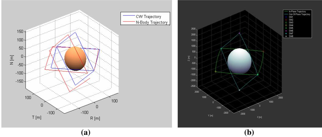
**Figure 10. Waypoint-based relative motion trajectories about a NEO (a) showing both linearized dynamics motion and non-linear dynamics motion including NEO gravity<sup>7</sup> and (b) showing only linearized motion and waypoints<sup>8</sup>.**
