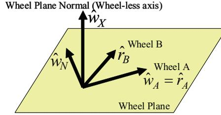
**Figure 4 Wheel-Orthogonal-Frame (WOF)**
