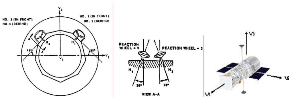
Figure 1 Reaction wheel assembly configuration
